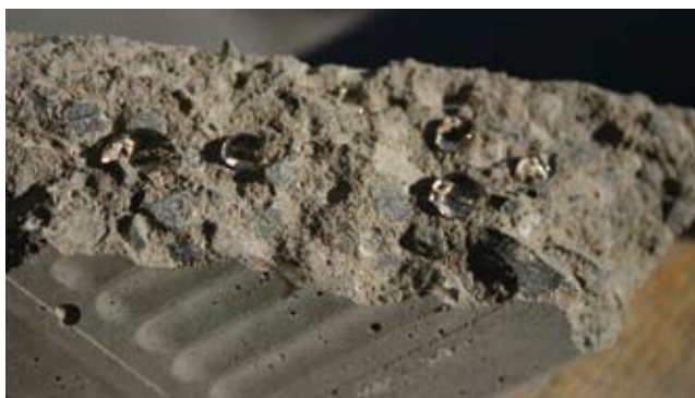
Photo 3. Concrete treated with a nanotechnology-based sealer repels water. Efficacy with friable mortars such as paving beds is not yet known.
